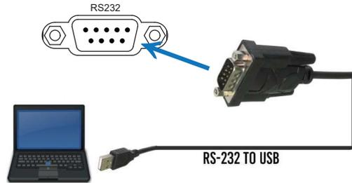
Then, open a Serial Command tool on PC to send ASCII command to control the Matrix.
